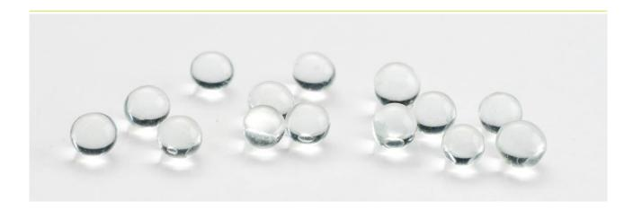
GLASS BEADS are fine blasting and reusable abrasives in accordance with DIN 8201, based on molten sodium glass. The product meets the work protection requirements in accordance with DGUV rule 100-500, part 2, chapter 2.24 "Working with blasting equipment (blasting work)".
