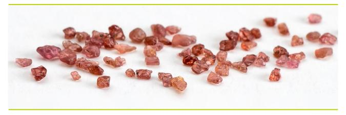
Garnet is a reusable mineral abrasive based on the natural occurring mineral Almandine. Garnet meets the requirements laid down in DGUV rule 100-500, part 2, chapter 2.24 "Working with blasting equipment (blasting works)."
