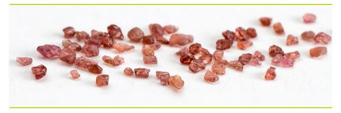
Garnet is a mineral cutting and filter media based on the natural occurring mineral Almandine. It is characterized by its high hardness and high specific weight. Due to the high hardness and cubic shape Garnet is perfectly suited as cutting media for waterjet-cutting-technology.
